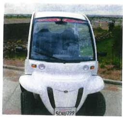
"The GEM (Global Electric Motorcar) is manufactured in Fargo, North Dakota and sold by Chrysler dealers. It is a street legal electric vehicle with 3-point seat belts, safety glass windshield, head and tail lights, turn signals, four wheel hydraulic brakes, independent front suspension, 72-volt motor, six 12-volt batteries, approximate driving range is 30 miles on one charge."
